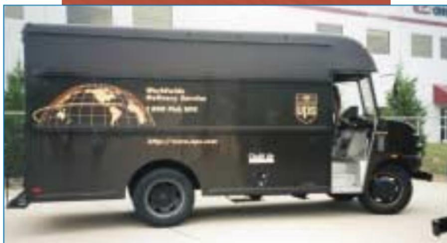
UPS delivery van powered by compressed natural gas (CNG)
