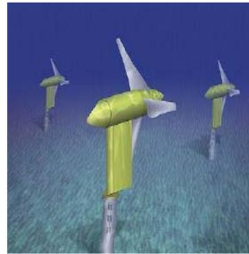
$$(P/A)_{\text{flow}} = 0.5 \text{ density } V^3$$
