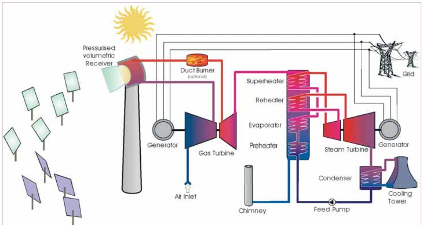
Figure 10 Schematic of a combined cycle system powered by a volumetric central receiver using pressurised air as heat transfer fluid (Source: DLR)
