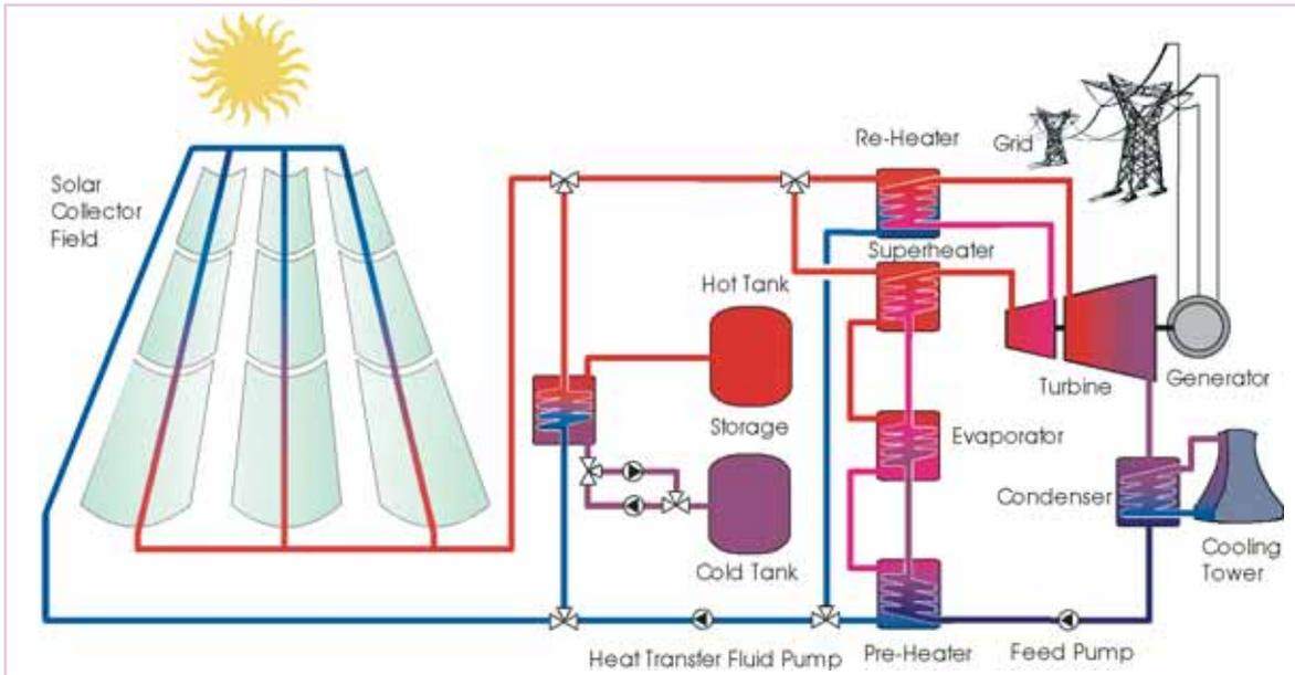
**Figure 2 Schematic diagram of a steam cycle power plant with a parabolic trough collector and a thermal energy storage**
