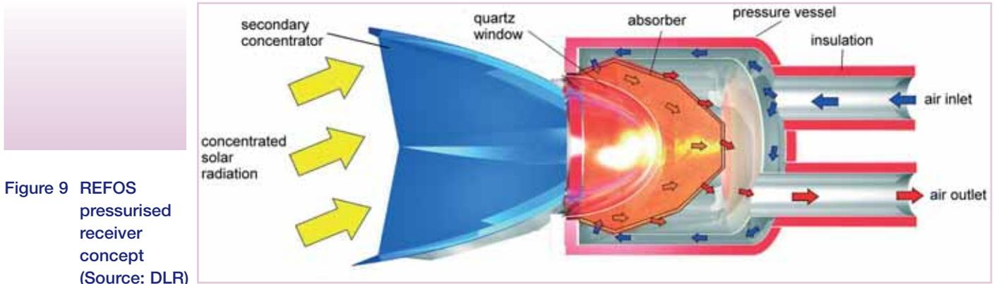
Figure 9 REFOS pressurised receiver concept (Source: DLR)
