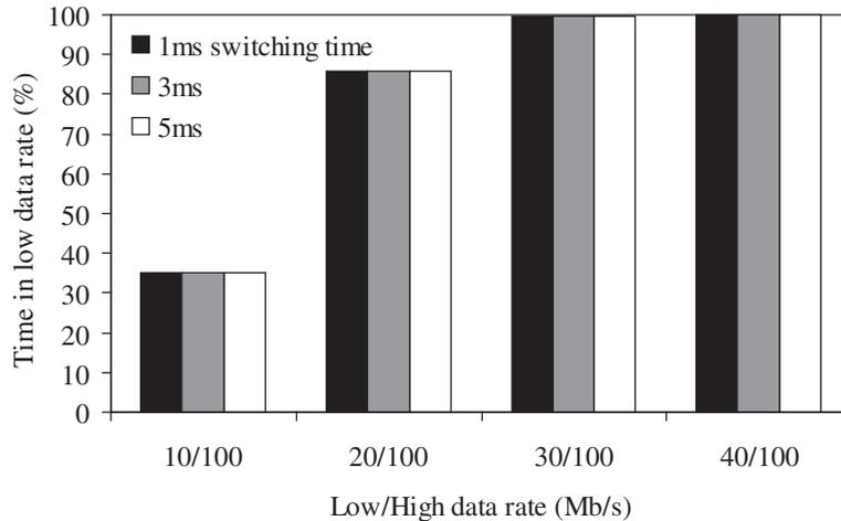
Figure 6. Time spent in low data rate as a function of low/high link rates
